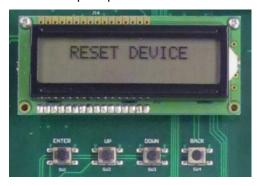
The cover of the transmitter must be removed in order to access the reset switch. Press the reset on the transmitter
