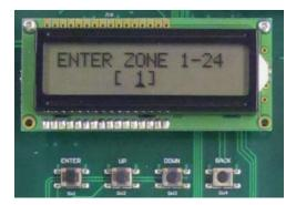
Enter the zone number that you wish to assign the transmitter from 1 to 32. Use "Up" or "Down" to change transmitter number.
