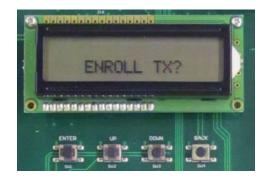
To begin enrolling transmitters, with "ENROLL TX?" being displayed on the LCD, press "ENTER"
