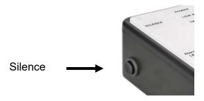
**Silence:** If pressed when any zone is in alarm, Red LED flashing and Audible sounder on, the audible sounder will turn off and the zone Alarm Red LED will change from flashing to steady
